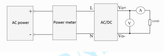
Figure 3-1 Single output product testing connection
