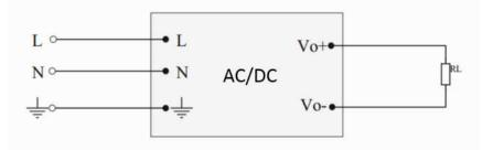
Figure 3-3 Application circuit diagram of conventional products
