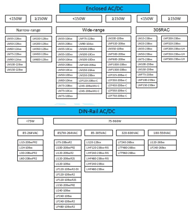
Figure 2-1 Enclosed/DIN-Rail AC/DC Selection Diagram
