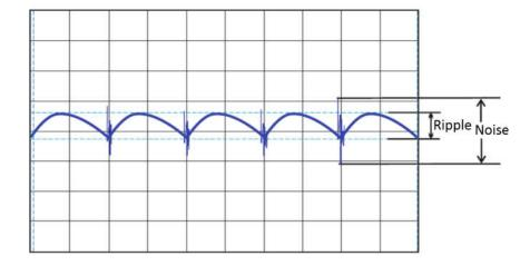
Figure 4-2 Waveform of Ripple and Noise Test
