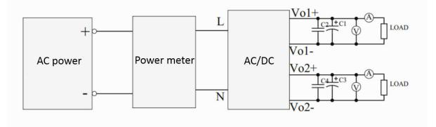
Figure 3-2 Multi-output basic test circuit connection
